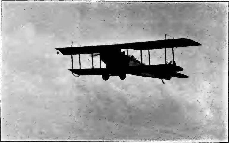
Fig. 8 —An Airplane viewed against the sky. In spite of the fact that the plane is painted white, it appears very dark when silhouetted against the bright clouds and sky.
